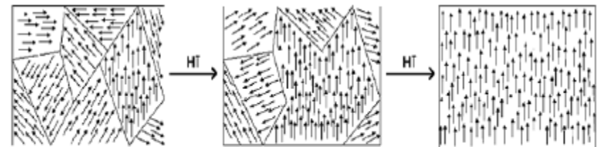
Figure 2 a – Resizing and reorienting of domains as a result of applied field H
