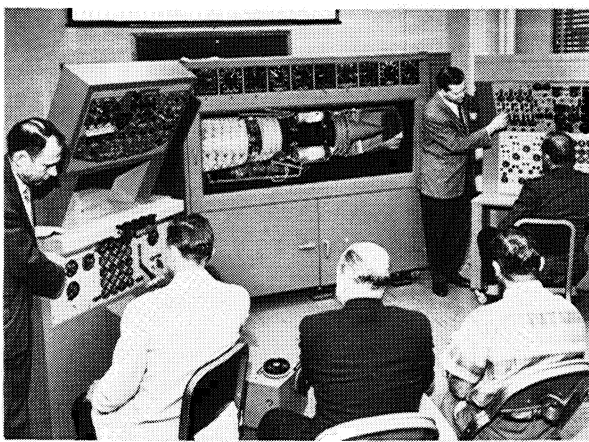
HOW DOES IT WORK? Realistic cutaway of jet engine, linked to pilot's controls (left) and flight engineer's controls (right) allow crew members to operate engine and read its performance as they would in airplane.
