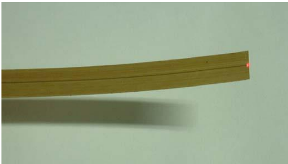
SMARTape Membrane Deformation Sensor
