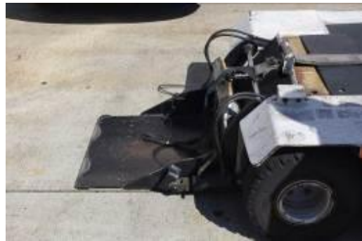
Figure 4: Lowered cradle on towbarless pushback
