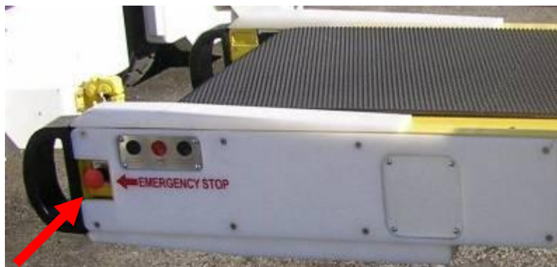
Figure 7 – Belt loader emergency stop button
