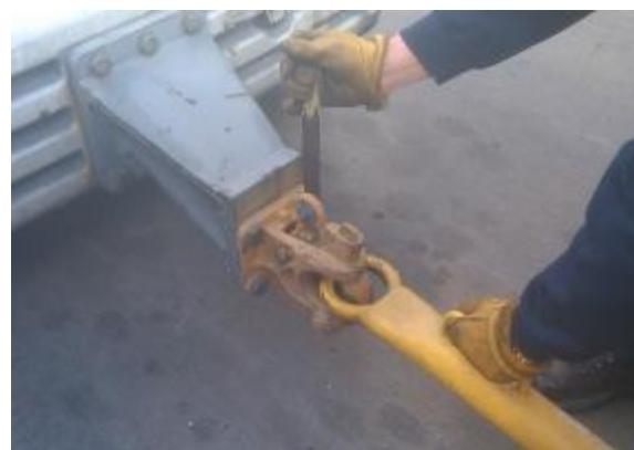
**Figure 7 - Always pull on hitch to ensure it will not open**
