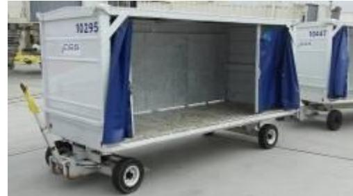
**Figure 9 - Always lock tongue in the upright position when left unattended**
