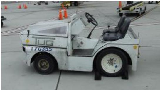
**Figure 1 - Correctly chocked vehicle**
