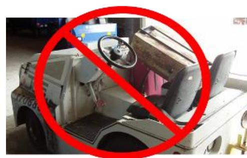
**Figure 2 - Never load baggage or freight in operator cabin**
