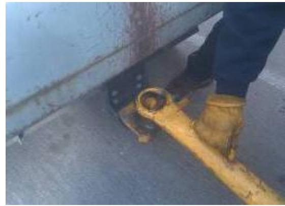
**Figure 4 - Pull on hitch to ensure tongue is secure**
